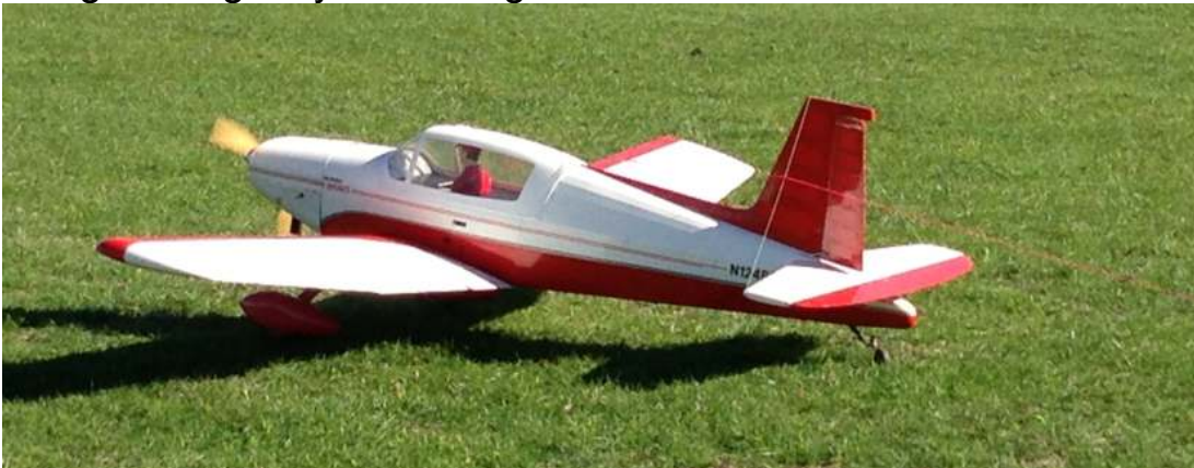
Pete's 40cc twin powered Morrisey Bravo. A fine tug for up 4.5m models. Looks good too!
